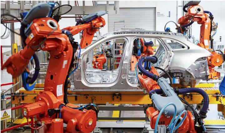
**Figure 1.2.** Robots in operation within an automobile factory. These processes are usually completely automated and controlled in real time. From *China’s robot market is still No. 1*, by ASIA TIMES ONLINE [Asi21].
